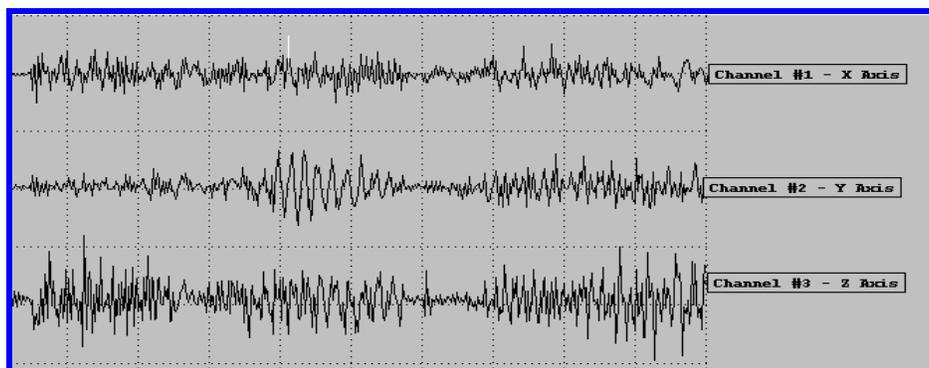
**Figure 2.** Expanded time history of one 6.5 sec recording. The highest acceleration levels are on the Z axis (vertical). The amplitude reached 20g's, peak to peak.
