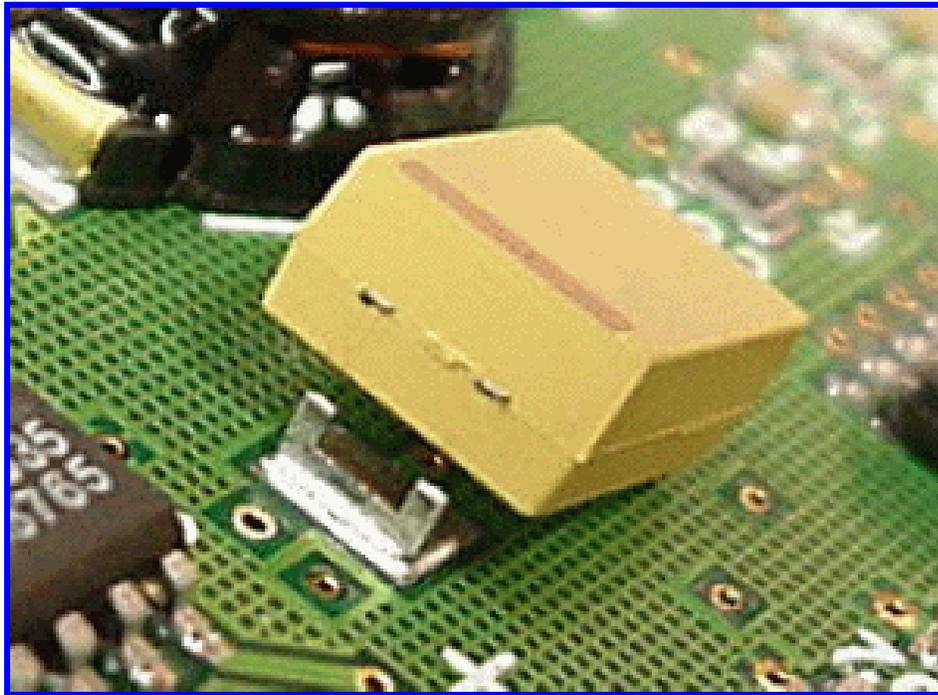
**Figure 5** View of failed surface mount capacitor. Failure was due to fatigue fracture accelerated by stimulus of router tool. Solder pad portion of lead is still connected to circuit board.
