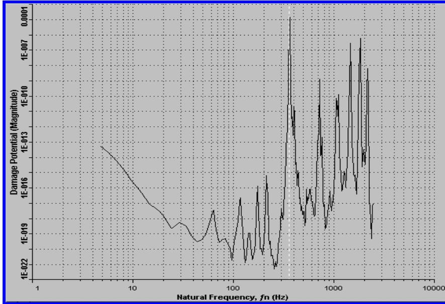
**Figure 4** The DP(f) for the complete routing operation for all four boards. The peak at 370Hz is 1.1E-4 DP units. Compare this to the mean of E-16.
