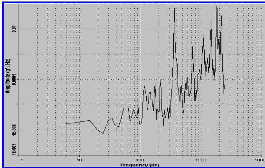
**Figure 3** PSD of Z axis acceleration created by router during PC board routing operation. The peak at 370Hz was obvious in all records.
