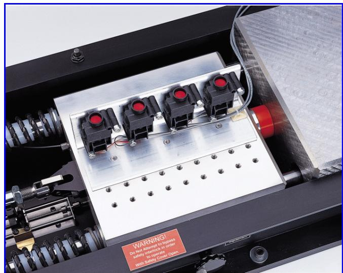
**Figure 2.** Table of shock machine for testing miniaturized products. On the table are car crash fuel shut-offs. Operation is also monitored.
