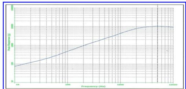
**Figure 4.** SRS of shock pulse seen in Figure 3. This shape is indicative of a classical half sine geometry shock.
