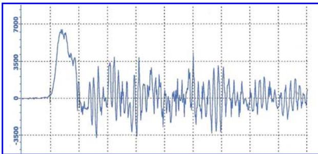
**Figure 3.** Shock amplitude is 6500g's, and the duration of the primary pulse is 200µsec. Ringing to the right of the primary is self resonance of either the fixture or the product itself.
