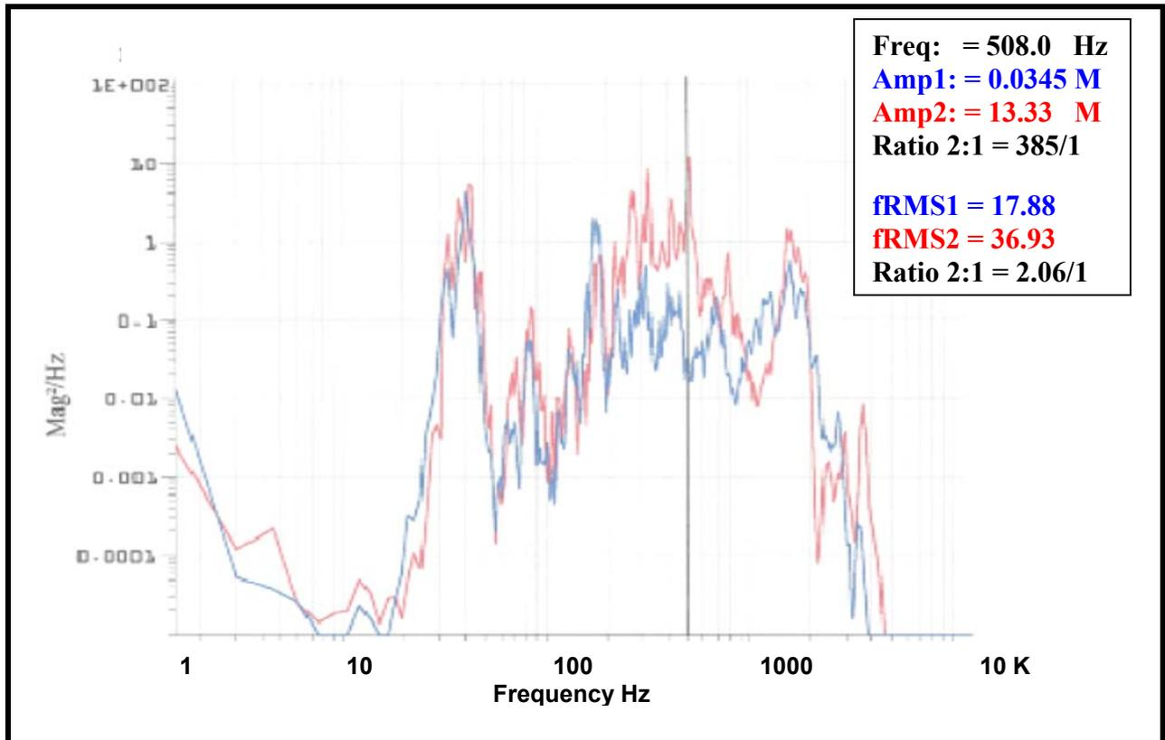
Figure 1. Overlaid DP(f) spectrums from two different 6DOF machines running at 10 gRMS.
