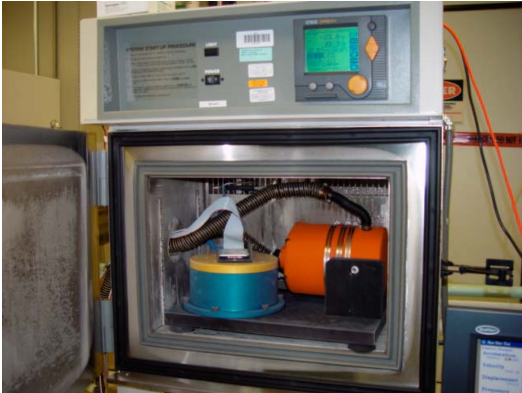
Figure 1. Environmental chamber with RVM-1 rotary table with hard disk drive mounted in the XY orientation.
