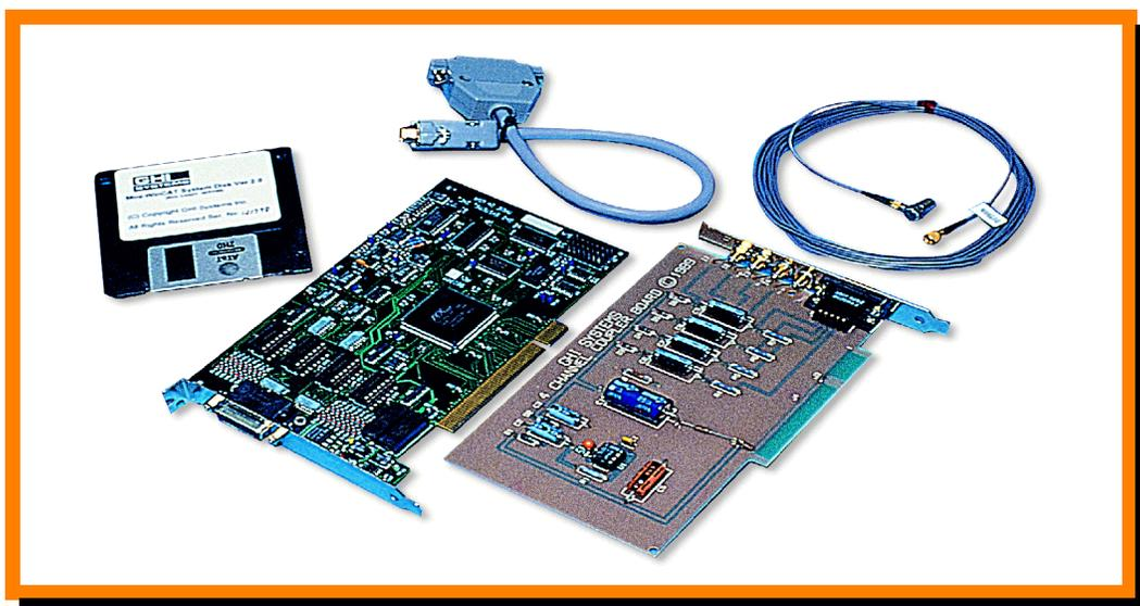
Figure 2. Typical WinCAT card and software set. Includes PCI bus analog amplifier and Digitizing Card, half ISA slot 4 Ch voltage mode sensor signal conditioner, software loader floppy, interconnect cable between digitizer and conditioner cards and accelerometer (furnished only with P/N 110-04 for protective package engineering tests). Note shown, 4 channel BNC DC sensor input box and its associated connection cable.
